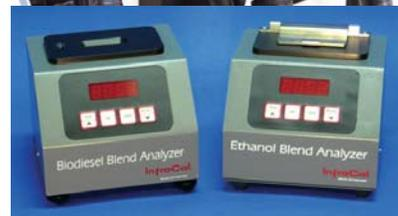
On-site analysis with InfraCal® Analyzers offers a quick way to verify that fuel blends are on spec. Incorrect blends can lead to regulatory fines, loss of customer confidence, and damage to equipment using the fuel.
